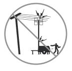
Keep away from the machine if it contacts energized power lines. Personnel must not touch or operate the machine until energized power lines are shut off.
