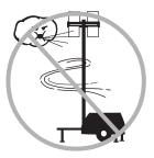
Do not raise the mast when wind speeds may exceed 62 mph / 100 km/h. Do not alter or disable machine components that in any way affect safety and stability.
