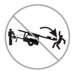
Do not remove batteries from the battery compartment unless all outriggers are lowered and in firm contact with the ground.
