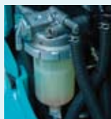
Pre fuel filter with built-in water separator
