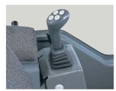
Automatic transmission is used with joystick steering.
