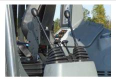
Mechanical controls can be ordered with Backhoe or ISO control patterns. Outrigger levers are conveniently located between the backhoe controls.
