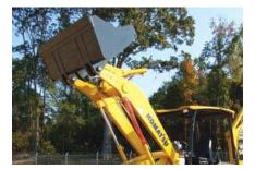
Bucket automatically self levels as the loader arms are raised.
