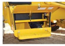
Lockable toolbox provides secure storage for tools, grease gun, etc. Also allows access to battery and hydraulic filter.
