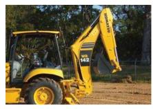
S-shape backhoe enhances truck loading and provides strong breakout and lift capacities.
