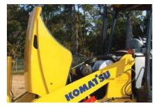
A tiltable engine hood allows access to service check points and can be locked with the ignition key.
