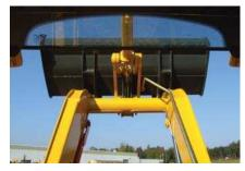
Front roof cutout provides a clear view of the loader bucket, even at maximum height.
