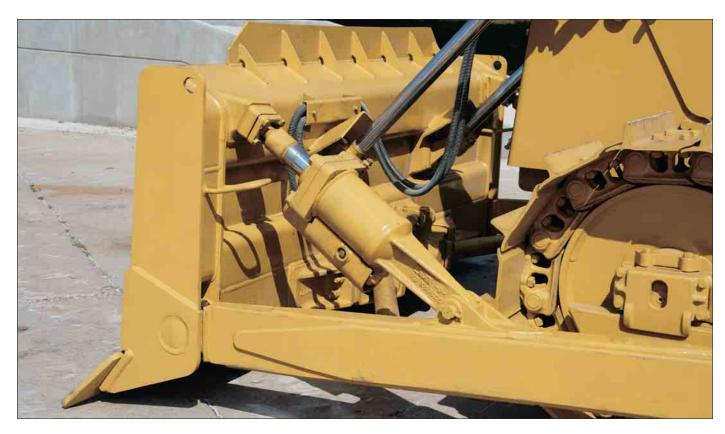
**Bulldozers.** All blades feature a strongbox-section design that resists twisting and cracking. Blades are made of Cat DH-2™ steel that has high tensile strength and stands up to the most severe applications. Heavy moldboard construction and hardened bolt-on cutting edges and end bits add strength and durability.
