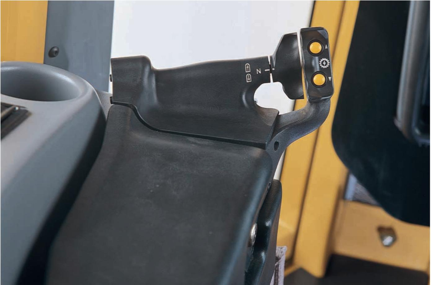
**Five Speed Forward/Reverse Gear Selection.** Five speed forward/reverse gear selection is achieved simply by pressing the yellow speed selection buttons. These buttons are integrated into the Finger Tip Control group.
