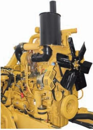
**Cat 3126B Engine.** The Cat 3126B engine is designed for easy maintenance and can be rebuilt for additional service lives. With the HEUI™ fuel system, injection pressure is independent of engine speed and provides maximum fuel delivery efficiency with low emissions.
