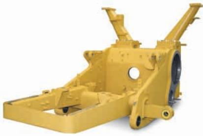
**Frame and Castings.** The D5N case and frames are built to absorb high impact shock loads and torsional forces. Castings are strategically located within the frame to add additional strength. Caterpillar uses robotic welding techniques in the assembly of the case and frames. This ensures quality and reliability throughout the structure.
