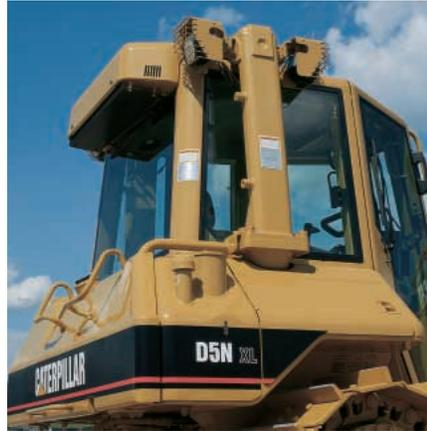
**Roll Over Protection System.** N-Series cab supports have been stiffened. Stiffer cab supports result in lower noise and vibration in the cab, providing the operator increased comfort.
