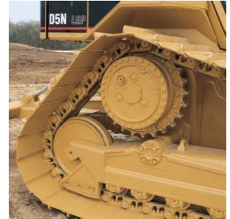
**Elevated Final Drive.** Final drives are isolated from ground and work tool induced impact loads for extended power train life.
