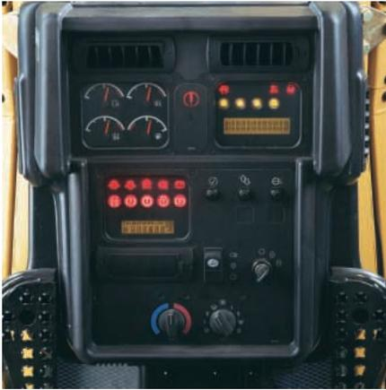
**Dash.** The instrument panel, with easy to read analog gauges and warning lamps, keeps the operator aware of any potential problems. All gauges and readouts are easily visible in direct sunlight. HVAC controls and vents are conveniently located on the dash to provide climate control for the operator. Auto-shift and Auto-kickdown controls are located within easy reach. Footpads keep the operator stable and comfortable while working on slopes.
