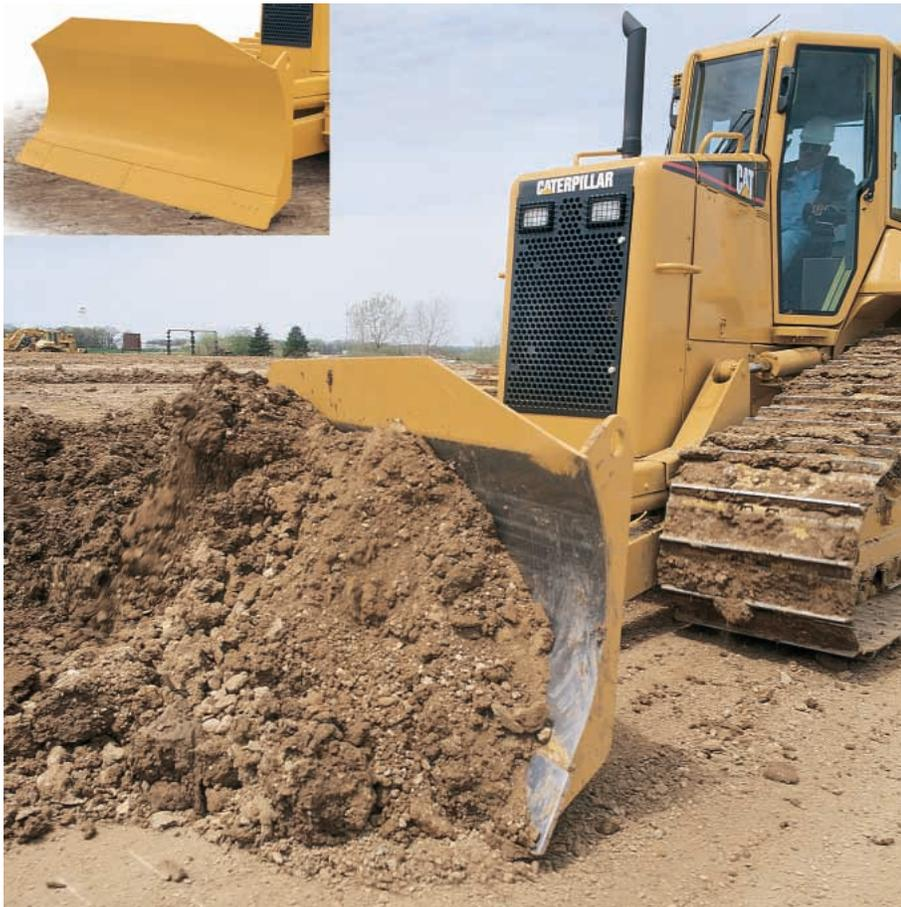
**Caterpillar Blades.** With superior moldboard and 4-cell structure design, Cat bulldozer blades hold up to the toughest job conditions. Our high-tensile strength blades resist torsional bending and deflection in tough applications.
