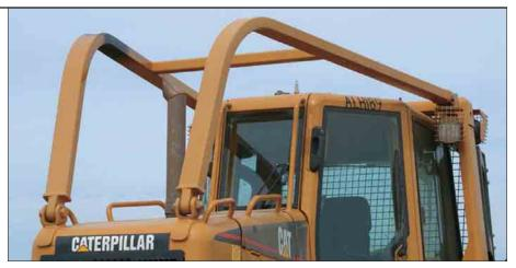
Forestry Sweeps. In forestry and land clearing applications where limbs and debris can damage a machine, optional sweeps are available for the N-Series. Sweeps help to shield critical components on the tractor such as hydraulic lines, exhaust stacks, cab windows and lights from damage.
