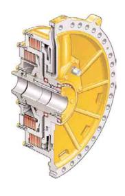
**Torque Converter.** The D5N single stage torque converter efficiently responds to changing load conditions by providing torque multiplication, therefore increasing drawbar power. It also provides protection to the drive train components by preventing shock loads from heavy dozing applications. This torque converter is efficiently matched to the power train components and provides the superior performance you need.
