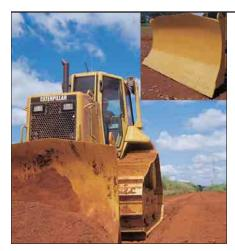
**Caterpillar Blades.** With superior moldboard and 4-cell structure design, Cat bulldozer blades hold up to the toughest job conditions. Our high-tensile strength blades resist torsional bending and deflection in tough applications.
