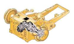
Frame and Castings. The D5N case and frames are built to absorb high impact shock loads and torsional forces.
