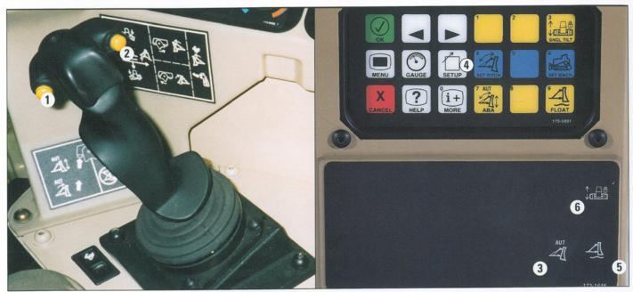
**Automated Blade Assist (ABA)** is a semi-automatic dozer control function that increases efficiency and reduces operator workload by automating some of the more common blade functions. The ABA system for a dual-tilt tractor consists of AutoPitch.
