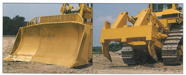
**Bulldozers.** The 11SU blade, rated at 27.2 m<sup>3</sup> (35.5 yd<sup>3</sup>) and the 11U blade at 34.4 m<sup>3</sup> (45.0 yd<sup>3</sup>) make full use of D11R power.
