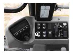
**Starting System.** The Electronic Speed Selector Switch (A), a "rocker" switch located on the right console, sets the engine rpm. The ADEM A4 engine controller will always start the engine in low idle. The engine rpm can be seen on the digital display of the instrument cluster in the gage cluster or in the performance menu in Messenger.
