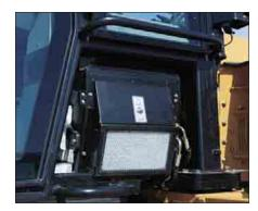
**Cab Air Filter.** The cab air filter, the grouped pressure taps, the cab tilt locking bar, the optional tilt cylinder and the tool box are conveniently located below the left-side cab window.
