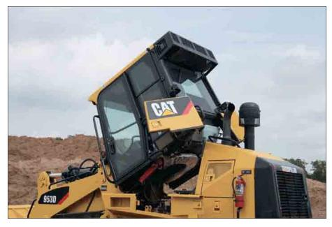
**Tiltable Cab.** The 953D is equipped with a tiltable cab. This feature makes the maintenance and the repairs easier. By tilting the cab, you can access to the drive train and perform complete service of the hydraulic system.
