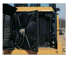
**Cooling System.** The fan and the grill swing open, providing excellent access for clean-out and maintenance. The heavy duty latched grill minimizes debris build-up.
