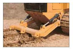
**Ripper-Scarifier**. A radial ripper-scarifier is available for the 953D as an attachment. It is mounted with two pins pressed into each side of the main frame. Two cylinders raise and lower the ripper. The ripper beam has three pockets for holding ripper shanks. The six pins in the linkage do not require lubrication. The 953D ripper-scarifier is intended for ripping frozen ground, asphalt and easily ripped rock. It is not designed for hard rock.
