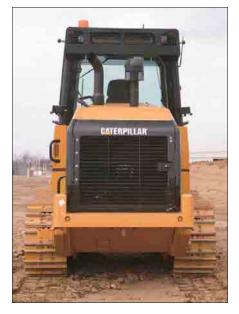
**Rear Engine Location.** Rear engine location allows excellent forward visibility, while serving as a working counterweight. It also helps reduce radiator plugging while providing easy service access to the engine and other major components.
