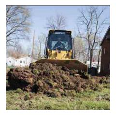
**Steering.** Steering is accomplished by changing relative pump flows and/or motor displacements, which causes one track to rotate slower than the other track. A more aggressive steering command (pushing one foot pedal down farther) will cause one track to stop/reverse while the other track continues to rotate.
