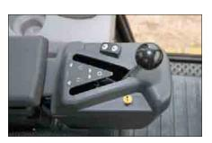
**Travel Speeds.** Travel speeds are infinitely variable between zero and top speed. Two speed modes "work" and "travel", provide two different speed ranges to best match machine speed and torque to the job conditions for maximum productivity. Maximum travel speed is 10 kph when the switch is set in the travel position.
