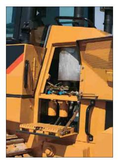
**Left side compartments.** Left engine compartment includes two spin-on hydraulic oil filters that provide filtration for the hydrostatic system. The lower part of the compartment door can be used as a step to access the shunt tank fill, the air pre-cleaner (if equipped) and allows easy cleaning of the rear window.
