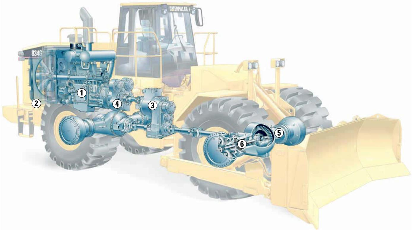
**1 Caterpillar 3456 Diesel Engine.** Is based on one of the most successful engines offered by Caterpillar, the 3406E. The 3456 is Tier 2 compliant and features increased horsepower and efficient fuel management for quick response, high productivity and exceptional service life. A new, sculptured cylinder block provides greater strength and is lighter weight.
