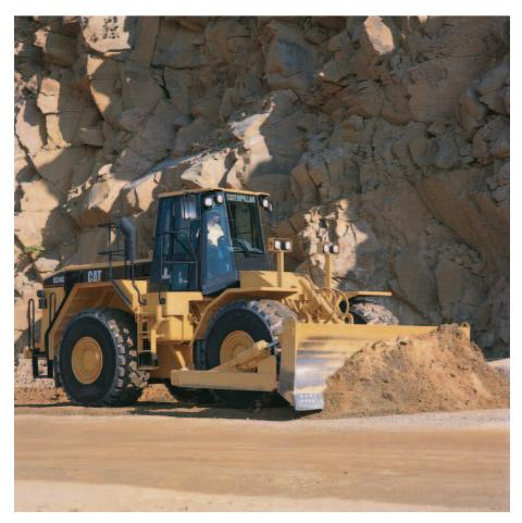
Woodchip U-Blade - with a unique wing configuration provides aggressive side setting into the chip pile, quickly knocking down stacked chips and loading the blade.  Extreme Service U-Blade - is designed for moving large loads over long distances in harsh conditions.
