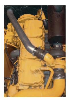
**Caterpillar 3406E Engine.** Is a six-cylinder, turbocharged, air-to-air aftercooled (ATAAC), Electronic Unit Injection (EUI) engine and one of the most developed and proven engines offered by Caterpillar. It has a strong reputation for reliability, durability and performance.
