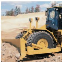
**Dozer Front Frame.** Built specifically to handle greater amounts of rimpull, the machine can readily push its weight plus the weight of the material for long distances in heavy dozing applications.
