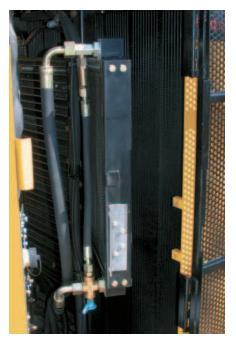
**Hinged Hydraulic Oil Cooler.** Can be swung open 30 degrees without special tools.
