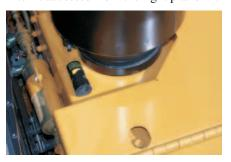
**Air Filter Restriction Sight Gauge.** Is visible from the cab or platform.
