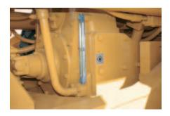
**Transmission Oil Fill Tube.** Is located beneath the platform area and the transmission oil dipstick has a sight gauge next to the fill tube for easy maintenance.
