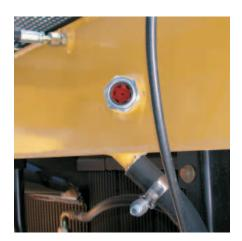
**Daily Maintenance.** Lockable ground level service doors give quick access to engine oil fill and dipstick, coolant sight gauge (above), rear frame grease fittings, relay panel and electrical breakers.
