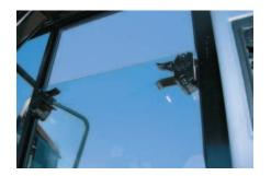
**Optional Sliding Cab Windows.** Are located in the right and left doors to provide access to outside air without opening the door.
