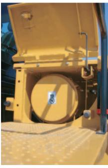
**Filter Access.** Is from the left platform for the primary filter, while the engine oil filter is accessed from the right platform.
