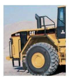
**Full Coverage Rear Fenders.** Extend to the bumper, along with a rear rubber (lateral) fender extension to ensure the entire tire width is covered.
