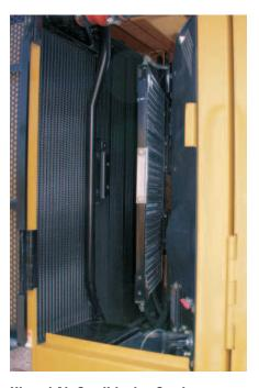
Hinged Air Conditioning Condenser. Swings open 30 degrees, and coupled with the swing out oil cooler allows the cooling system to be cleaned quickly and easily.
