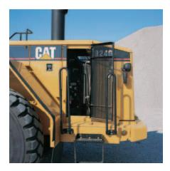
**Separated Cooling System.** Isolates the fan and radiator away from the engine for a quieter running machine. AMOCS reduces radiator repair time. The new metal engine enclosure is completely redesigned for greater durability and to provide easy access for daily maintenance and inspection.
