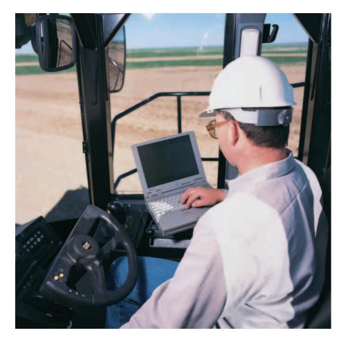
Caterpillar Monitoring System. Provides diagnostics that allow technicians to review a machine's operation and quickly troubleshoot problems. Operating parameters, diagnostic codes and out-of-range gauge readings are displayed through the diagnostic connector. There are also pressure taps for easy hydraulic system checks.
