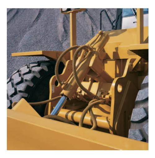
**Hydraulic System.** Provides low-effort blade control. Seat-mounted levers send electrical signals to a pilot valve mounted on the front frame. This moves the sound, heat and effort caused by a hydraulic valve out of the operator's station.
