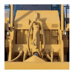
Optional Counterweight. Is located on either side of the front frame. For each specific application there is a correct machine weight for proper balancing of traction, floatation, mobility and response. Lower machine weight is usually required for typical second gear applications such as fill spreading, stockpiling, road maintenance, towing implements and shovel cleanup. Higher machine weight is usually required for such typical first gear applications as heavy dozing and pushloading.
