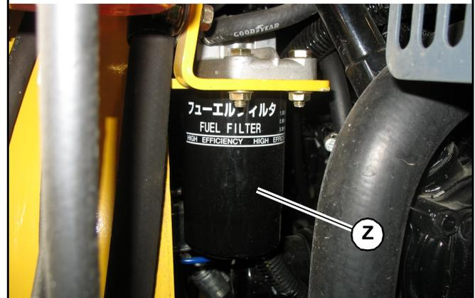
Fig. 142 – Engine Fuel Filter
