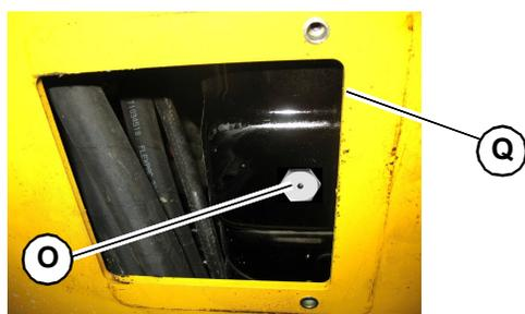
Fig. 127 – Engine Oil Drain Plug (Later Models RT175/RT210 Shown; RT250 Similar)
