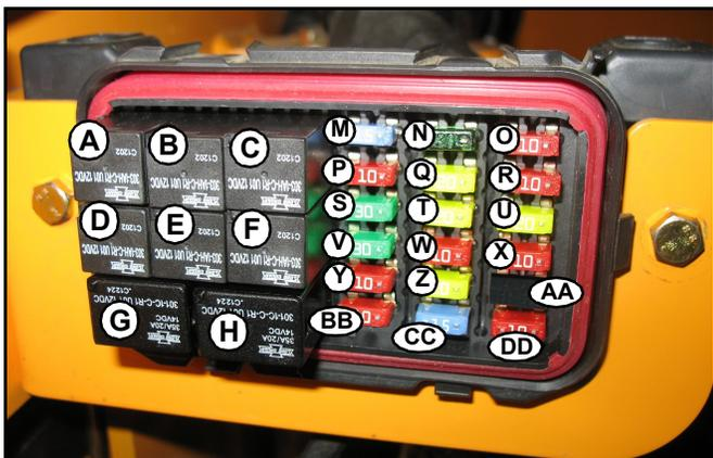
Fig. 164 – RT250 Fuses – Engine Compartment
