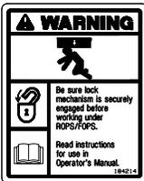
(Located on the bottom of the ROPS / operator's platform and to the left of the rear cab window just above the ROPS tilt lock.)
