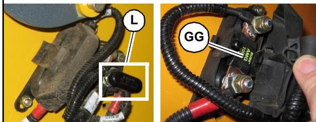
Fig. 167 – RT250 Power-A-Tach®, Glow Relays / Fuses
