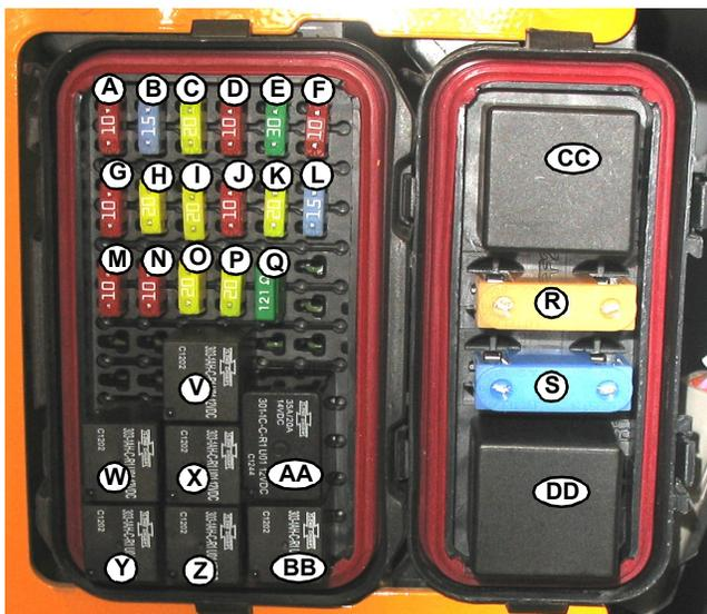
Fig. 168 – Fuses – Engine Compartment
