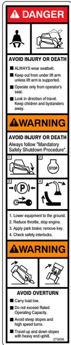
(Located on the inside of the right door pillar inside the cab)
