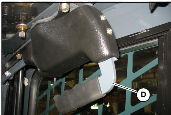
Fig. 49 – Closing the Door from the Inside
