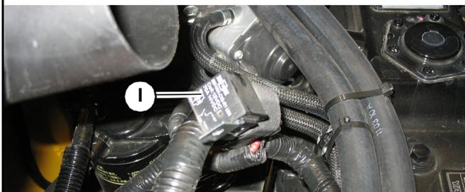
Fig. 172 – Engine Pre-heat Relay
