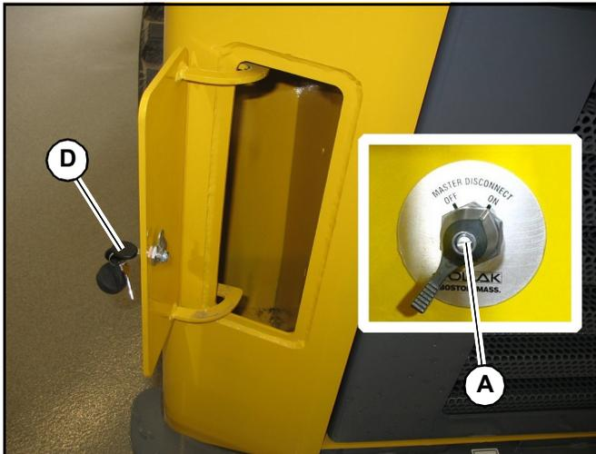
**Fig. 40 – Battery Disconnect Switch**
