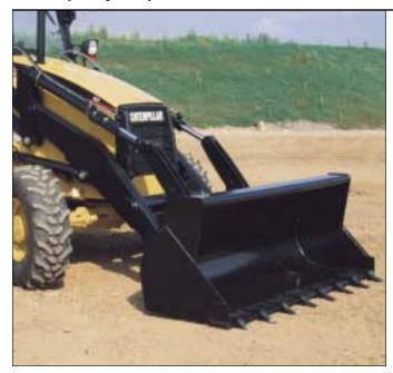
Loader. The parallel loader provides maximum lift and breakout forces, and parallel lift for efficient loading and material handling. A return-to-dig system makes operation easy, and improves cycle times. The optional hydraulic Quick Coupler provides versatility and allows quick connection to selected attachments available for the Cat family of integrated toolcarriers.
