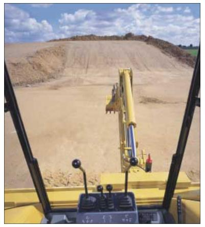
**Visibility.** The Cat 428C is specially designed for maximum visibility – all around. The sloping front hood and divergent lift arms allow the operator to see more of the forward work area and loader attachment. And there's no precleaner to look around. Rear visibility continues to be the best in the industry with a narrow boom and a rear window that stows above the operator out of view.
