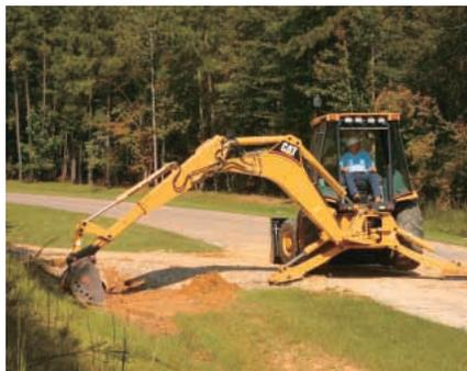
**Backhoe Boom.** The excavator-style boom features box section fabrication with internal stiffeners for better balance and weight distribution. The curved design provides additional clearance over obstacles while digging a trench or truck loading. The narrow boom enhances the viewing area to the bucket and trench throughout the entire operating range.
