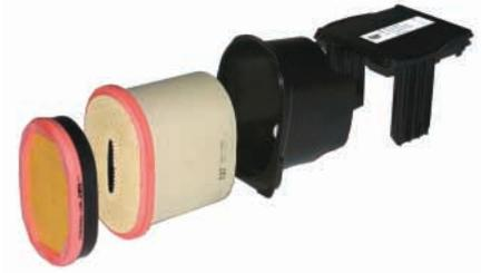
**Air Cleaner.** A new, dry-type, axial seal air cleaner with automatic, integrated dust ejection system provides more efficient pre-separation. The two-stage air filter incorporates both air cleaner and precleaner functions into a single unit mounted under the hood.
