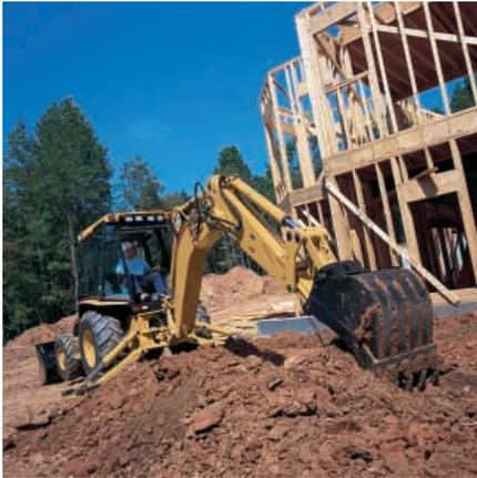
**Heavy Duty Rock Bucket.** Specifically designed to address harsh, rocky conditions and capable of digging in granite, caliche and rocky soil.
