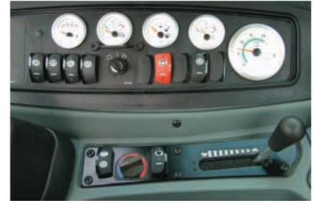
**Operator Controls.** The controls of the 420D/420D IT have been carefully laid out to create a user-friendly environment. Switches, boom lock and pilot operated stabilizer controls are located in the side console, within easy reach of the operator. White-faced gauges are easy to read and the low effort pilot controls reduce operator fatigue and help boost overall productivity.
