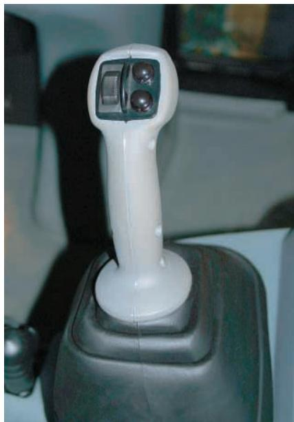
**IT Loader Controls.** The 420D IT has a new, standard single lever, pilot-operated loader control for proportional control and fine modulation of the hydraulic work tools. A thumb roller control on top operates auxiliary hydraulic functions such as the clam bucket and two buttons control hydraulic broom angle.
