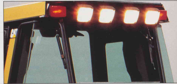
Lights like never before: Double the standard lighting capability with new optional front and rear arrays on B-Series units, for added nighttime visibility where and when you need it most; and roof extensions provide improved rain protection and help protect lights.
