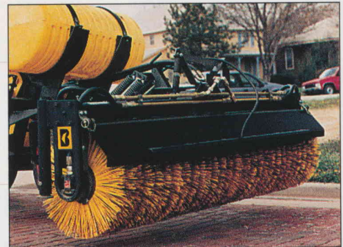
Sweep streets, parking lots and more when your loader bucket's replaced with a hydraulic broom—complete with water system.
